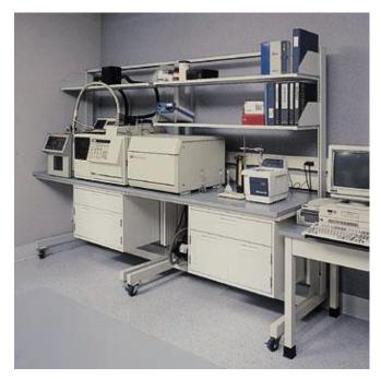
Strategies to build flexible, collaborative research environments include the use of casework systems that are easily moveable, limiting fixed elements in the laboratories, and containing hazards in the smallest workable area. Movable and height-adjustable laboratory benches with only minimal services are the norms in the interior of laboratories. Flexible engineering services—supply and exhaust air, water, electricity, voice/data, and vacuum systems—are extremely important to labs.
